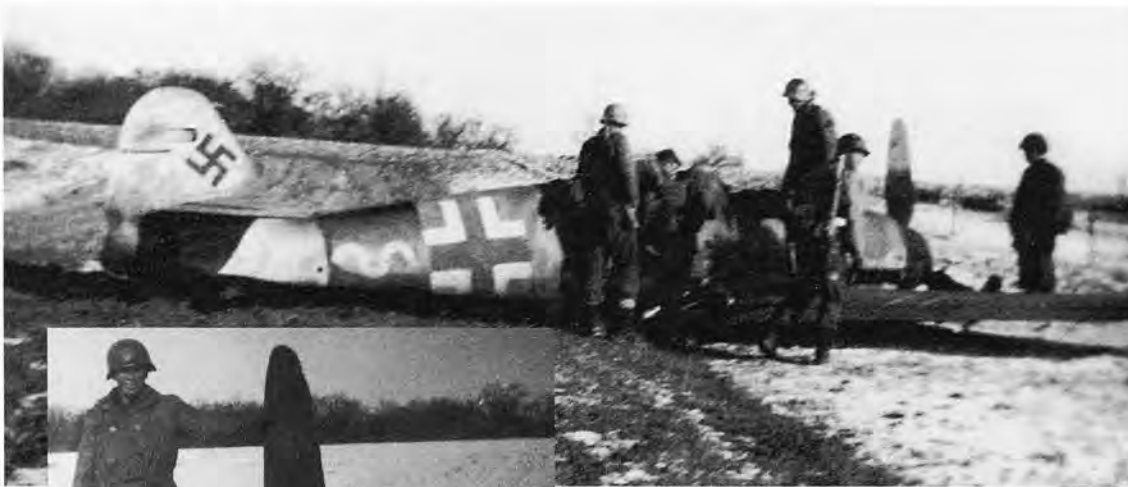
Gefr. Alfred Michel's 'Blue 2' being examined by US forces. Note that the propeller was already feathered when the aircraft belly-landed. (Williams)
