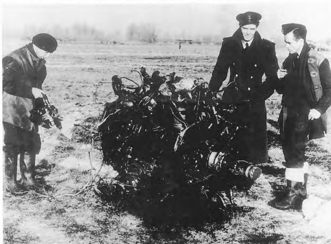
Polish airmen inspect the remains of a BMW 801 engine from one of the Fw 190s which crashed on St.Denis-Westrem airfield. Note the Spitfire in the background. (Delbaere/Hugot)
